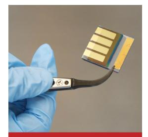
ABOVE: A CHIP WITH FOUR PEROVSKITE SOLAR CELLS MADE IN NITIN PADTURE'S LAB. THE CELLS WILL BE MOUNTED ON THE OUTSIDE OF A STUDENT-BUILT SATELLITE AND OBSERVED BY A BOOM-MOUNTED CAMERA WHILE IN SPACE.
