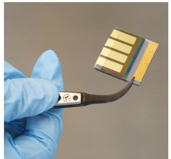
ABOVE: A CHIP WITH FOUR PEROVSKITE SOLAR CELLS MADE IN NITIN PADTURE'S LAB. THE CELLS WILL BE MOUNTED ON THE OUTSIDE OF A STUDENT-BUILT SATELLITE AND OBSERVED BY A BOOM-MOUNTED CAMERA WHILE IN SPACE.
